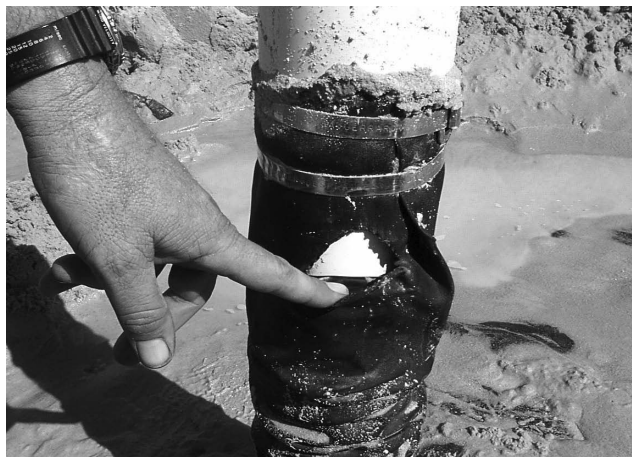
Figure 7. Bore casing at Oxy-02 (used to install oxygen probes below the composite cover), showing the tear in the composite cover near where it was attached to the bore casing.
